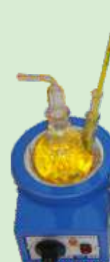
Condition of other synthetic Thermic Fluid, after heating 320°C
