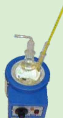
Condition of Hi Tech Therm S3 , after heating 326°C
