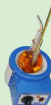
Condition of mineral oil after heating 300°C
